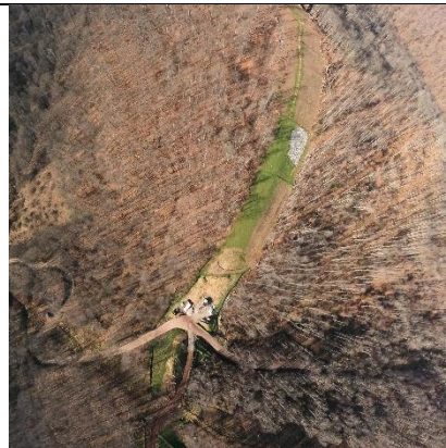
Milepost 56.5 G0024748.jpg Bare, unvegetated areas north of Brush Run Rd and farther uphill. Slip area shown midway up slope.
