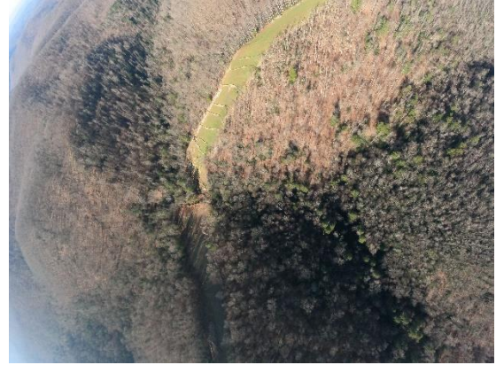
Milepost 79.7 G0024321.jpg Bare areas, looks like sediment may have washed out where they are trying to contain
