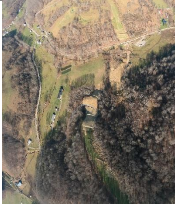
Milepost 44.8 G0024963.jpg Unvegetated areas and extensive matting south of access road to crossing of Fink Ck. Sediment appears to be in stream.
