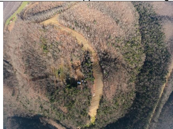
Milepost 74.6 G0024410.jpg Bare dirt. No vegetative cover in areas.
