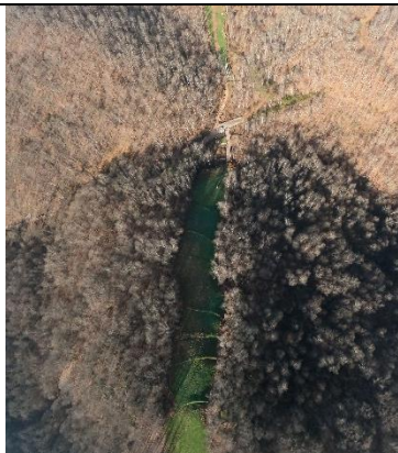
Milepost 61.3 G0024660.jpg Lack of vegetation next to stream crossing.
