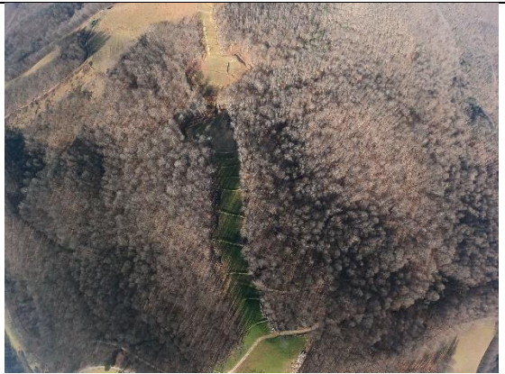
Milepost 78.2 G0024346.jpg Bare areas, lot of loose dirt by a stream crossing.
