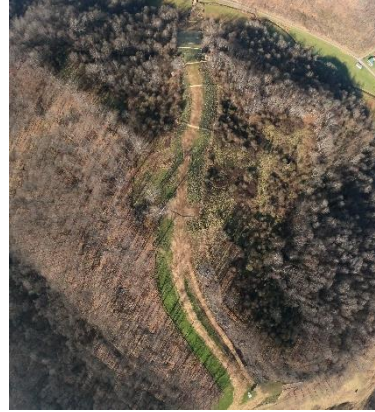
Milepost 58.7 G0024705.jpg No vegetative in ROW next to wetlands crossing.
