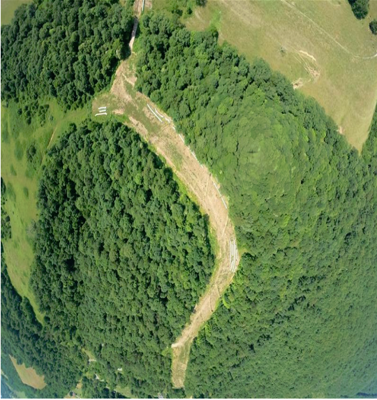
Milepost 172.3 Bare, exposed soil in ROW.
