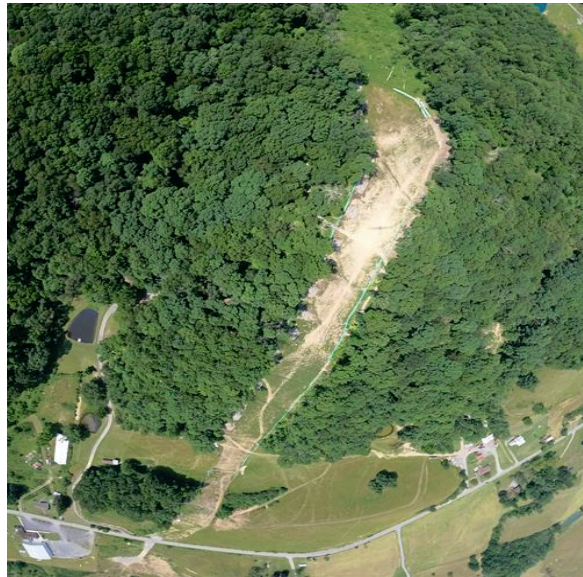
Milepost 191.3 Bare soil on slope does not meet adequate vegetative coverage requirements.
