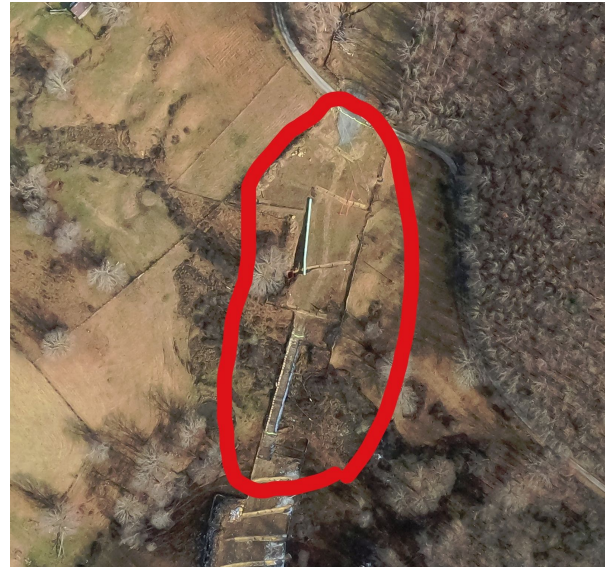
Milepost 106.4 G0023856.jpg Area on the slope above wetlands crossing is bare and needs vegetative stabilization.
