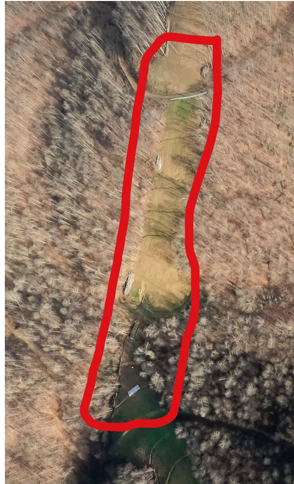
Milepost 90.7 G0024138.jpg Unvegetated areas adjacent to stream crossing on both sides. Inspection requested.
