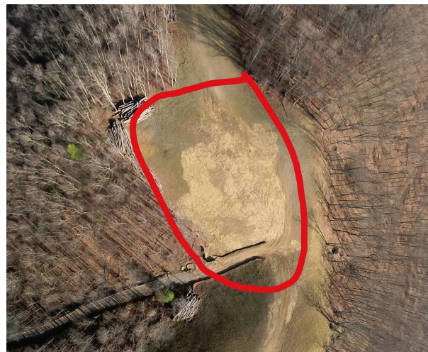
Milepost 83 G0024264.jpg Bare area on top of ridge. Additional seeding needed to cover the area.
