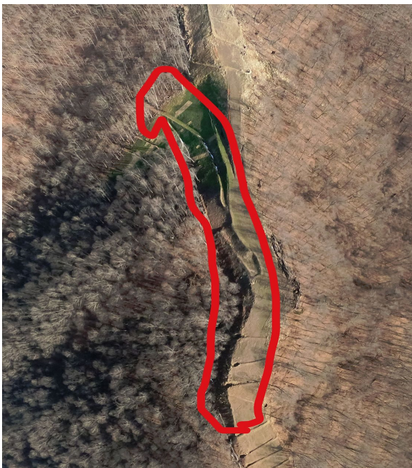
Milepost 86.9 G0024202.jpg Steep drop off, clear erosion/brown dirt on side of dropoff. Drainage channels forming on edge of ROW. Needs inspection.
