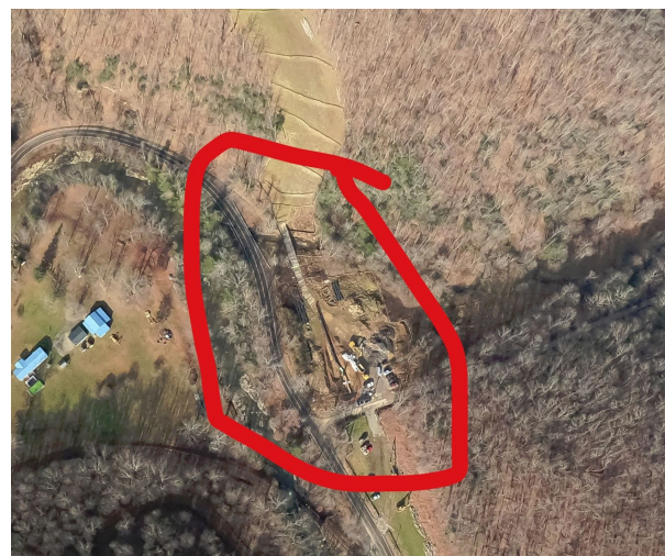
Milepost 98.7 G0023997.jpg Large area with little vegetation on both sides of stream crossing. Work area perimeter control is too close to the edge of the live stream. Inspection requested.
