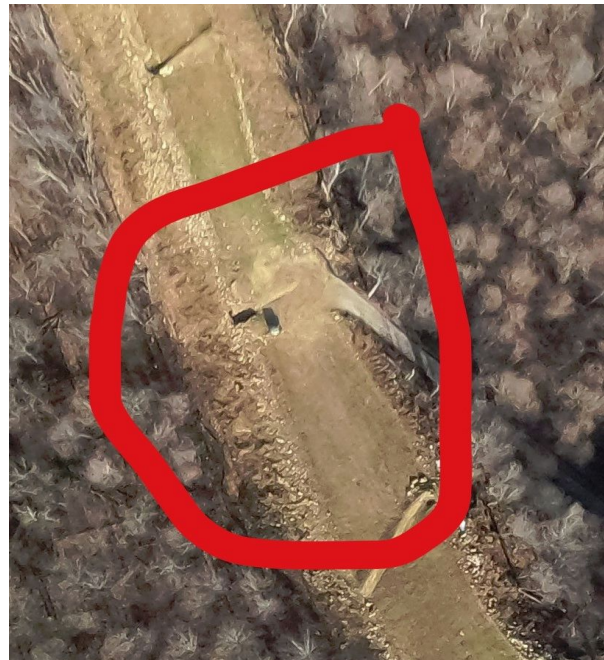
Milepost 94.3 G0024075.jpg Small area at low point/access road with sparse vegetation. Additional seeding necessary at this location.
