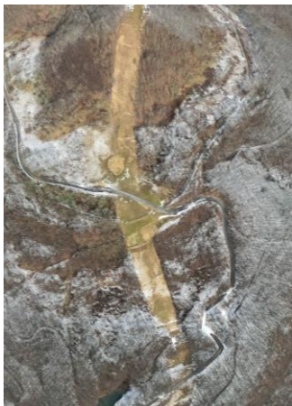
Milepost 141.6 G0023245.jpg Long slope with bare/sparsely vegetated areas. Re-seeding required.
