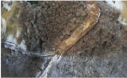
Milepost 156.4 - 156.5 G0022985.jpg Large area on slope at end of access road with sparse or dead vegetation. Slips and rill gullies forming on bare areas of slope.
