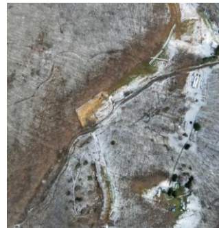
Milepost 140.8 G0023259.jpg Area next to the road crossing has no vegetative cover in place. Inspection needed to determine the condition of this area.
