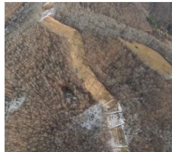
Milepost 153.75 - 153.9 G0023025.jpg Bare or sparse vegetation. Re-seeding is needed.
