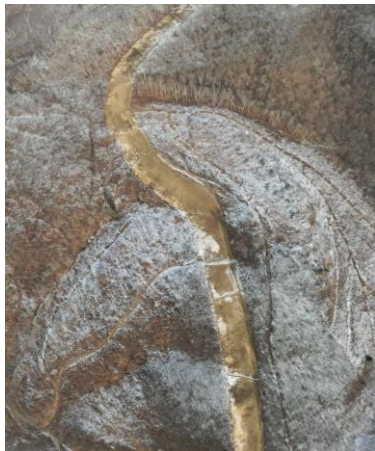
Milepost 141.6 G0023245.jpg Long slope with bare/sparsely vegetated areas. Re-seeding required.
