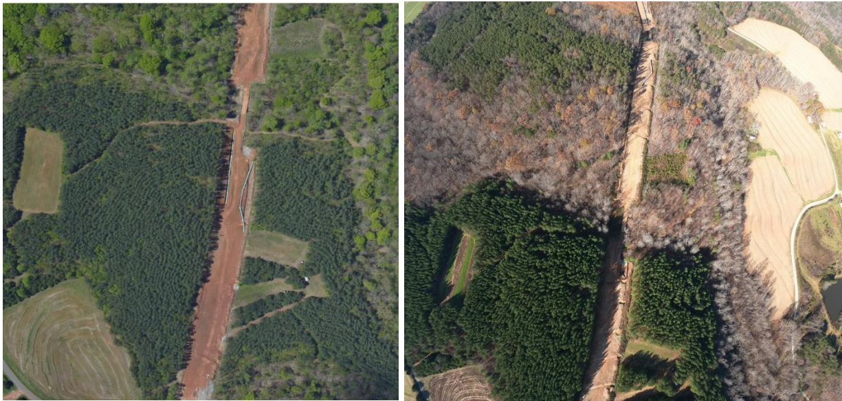
Milepost 294.8: Photo on the left was taken on April 21, 2019. Photo on the right was taken on November 21, 2020. Both photos show bare, uncovered areas with little vegetation. There is dead grass in parts of the photo taken in 2020, which does not meet vegetative cover requirements.
