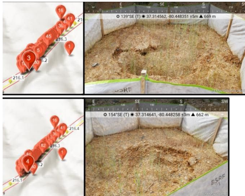
Figure 6: May 2019, two images showing more areas of subsidence enclosed in silt fence.
