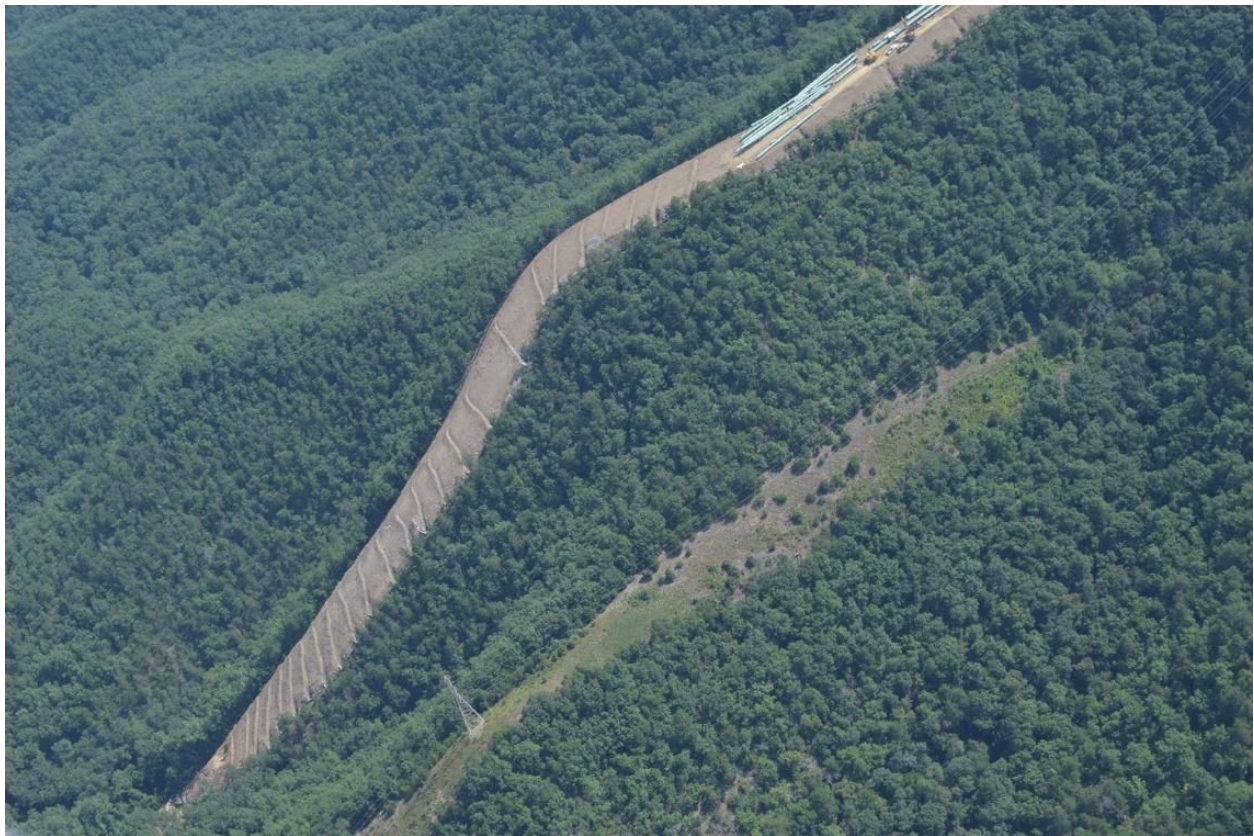
Figure 8. A July 27, 2017 flyover of the MVP ROW showed the magnitude of disturbance on steep slopes above Bradshaw Creek and other Roanoke River tributaries.
