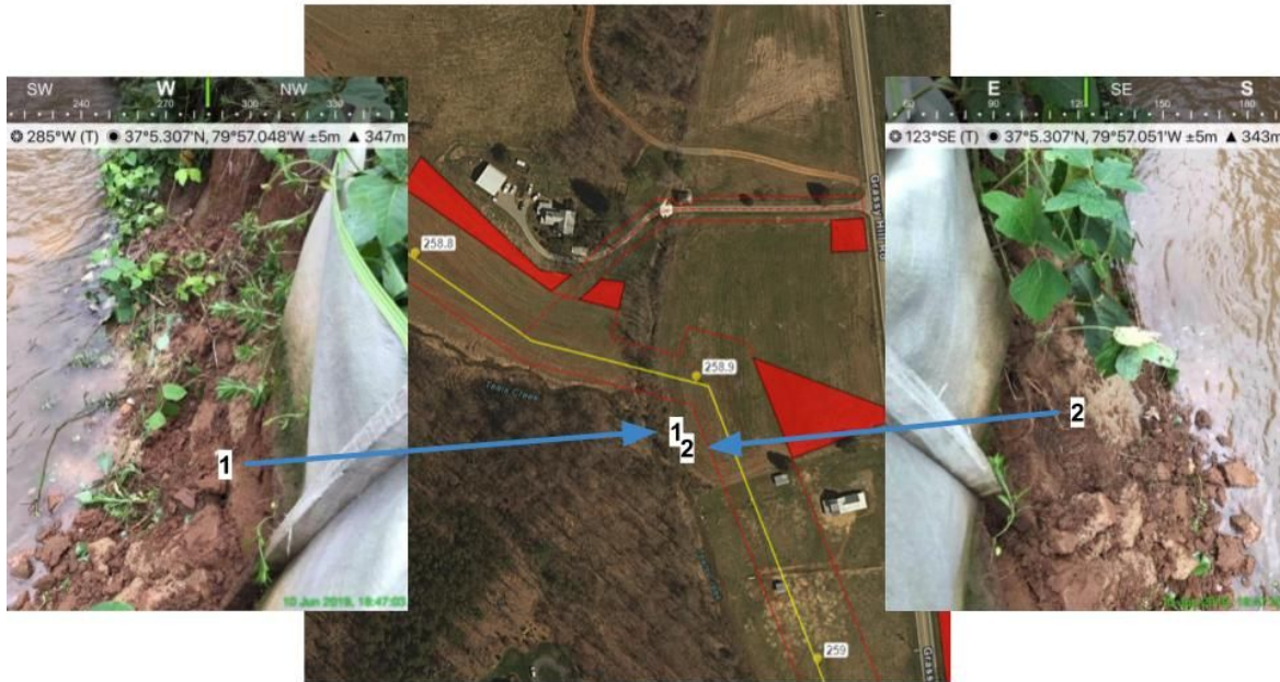
Figure 2: Stream bank scour is about to undercut the silt fence on Grassy Hill Road, 5/10/2019.
