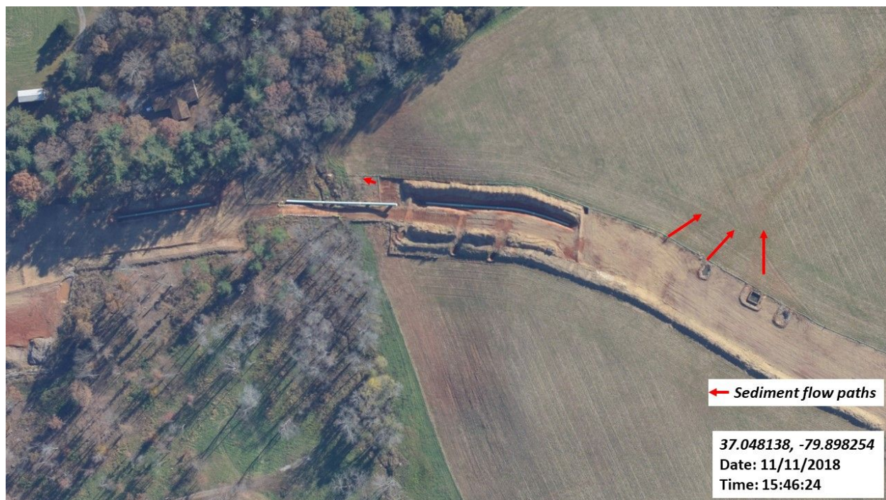
Figure 19: Sediment flowing into adjacent field.
