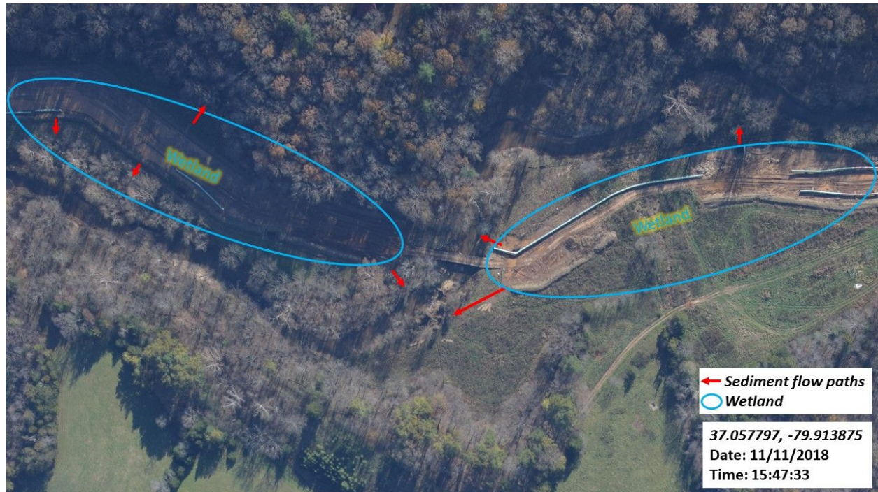
Figure 26: Sediment flowing off of right of way into stream and wetland areas.
