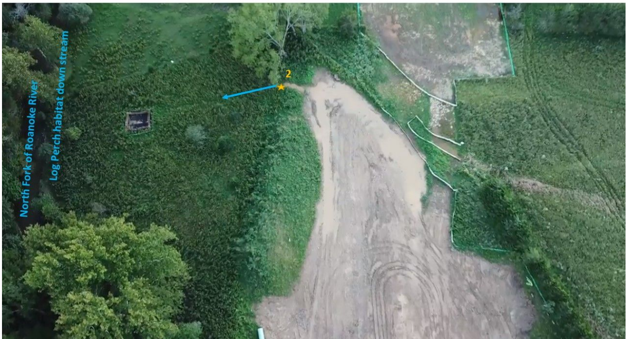
Figure 11: Location 2 is another location at this site where sediment laden stormwater continually flows into the North Fork of the Roanoke River during rain events.
