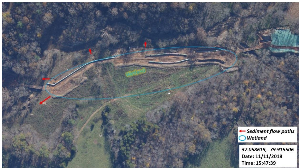
Figure 27: Trenching in a wetland; area is shown in ground photos below from table 1 & 2.
