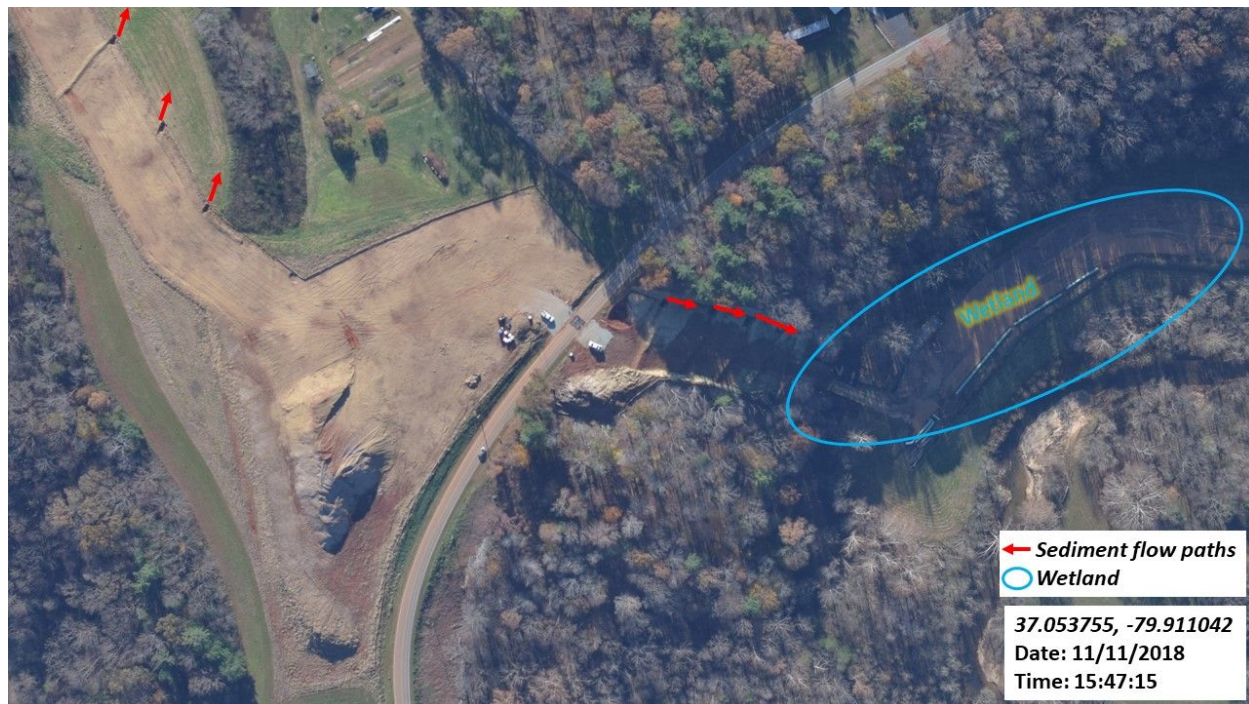
Figure 24: Iron Ridge Road shows discoloration from mud in roadway. Flow paths and wetland identified.
