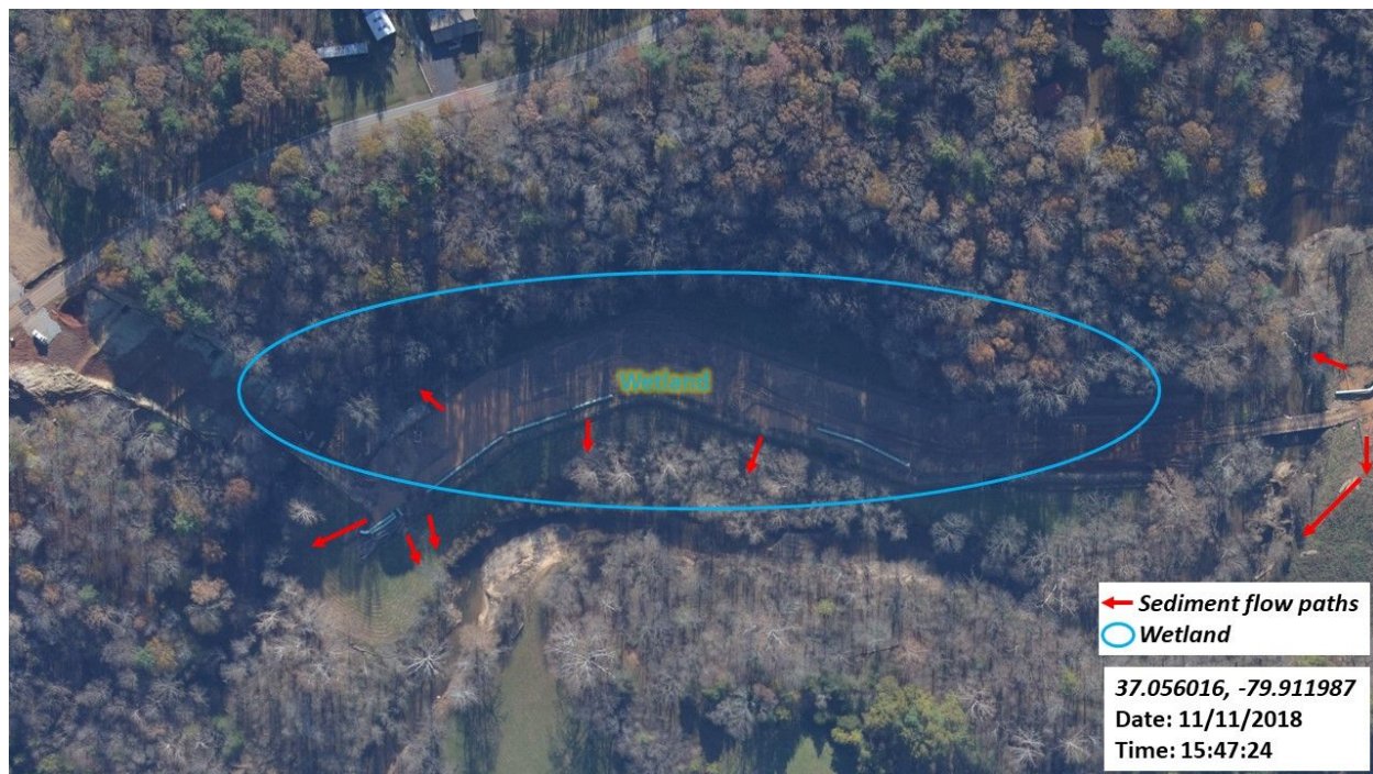
Figure 25: Sediment flowing off right of way into adjacent stream. Sediment deposits may be seen along stream.
