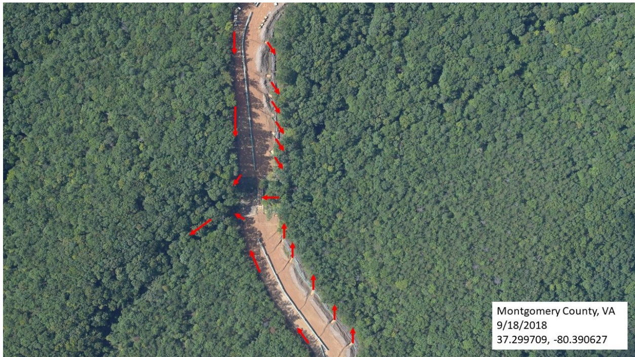
Figure 6: Brush Mountain in Montgomery County, Virginia; Flight date 9/18/2018; Flow lines indicated by red arrows.
