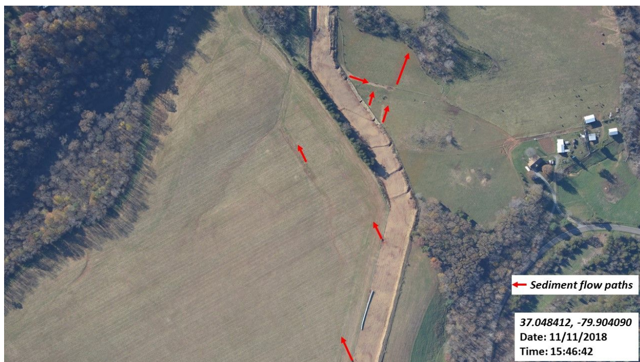
Figure 21: Sediment flowing into field from right of way diversions.
