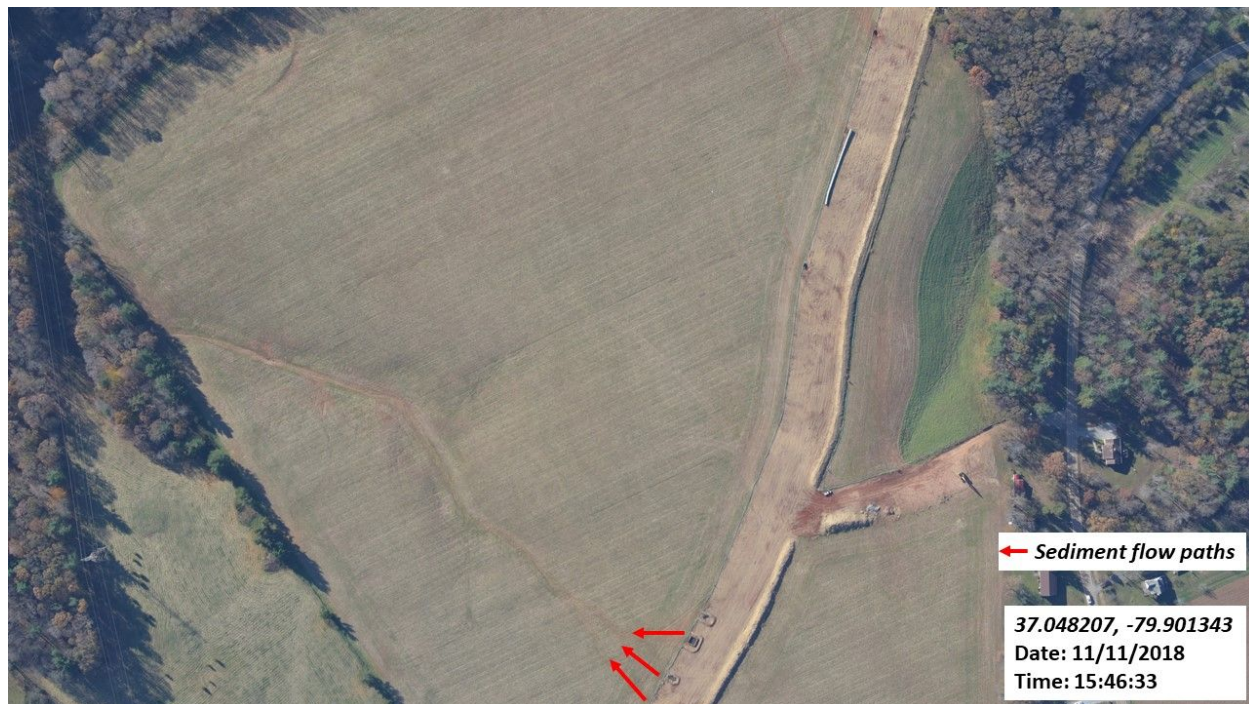
Figure 20: Sediment flowing into adjacent field into drainage channel conveying sediment to stream.
