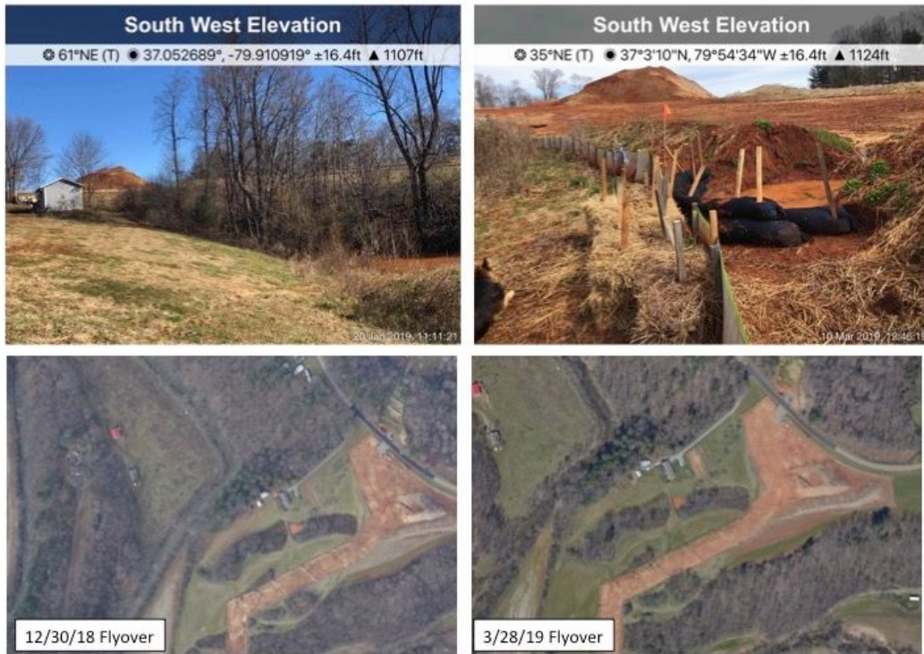
Figure 8: Ground and aerial images of unseeded earth pile on Angle property continuing through the winter months. Note pond filled with sediment mid-photo in the aerial images and bottom left in the January 20 ground image.
